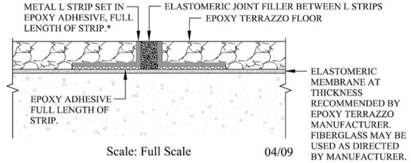
The use of divider strips (L strips) should be considered in areas where floor temperature changes may occur. Such as glass walls and or sky lights, if joints are to be used, the design teams must determine spacing.
